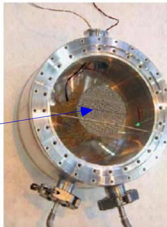
Array of heating wires for tests
