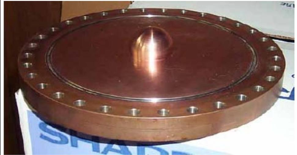
Note: electrode shape adjusted to tune resonance
