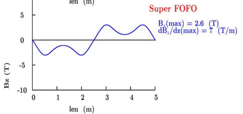
→ Periodic (alternating-gradient) focusing allows low  $\beta$  w/ much less superconductor
