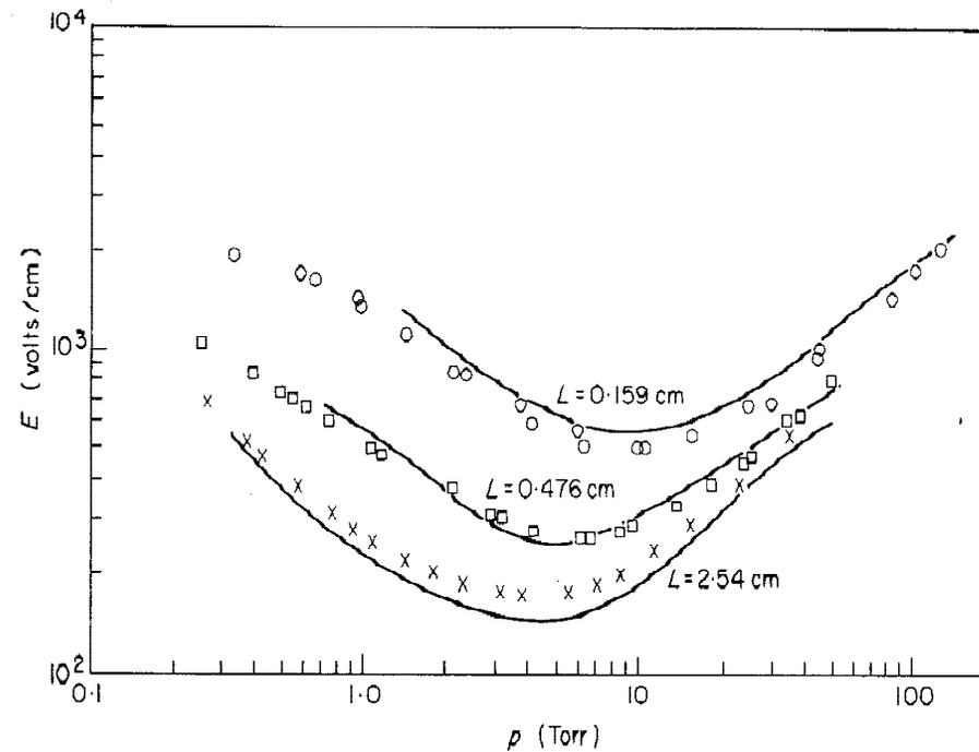
Breakdown voltages in hydrogen (Müller, 1966. permission of Springer-Verlag)
