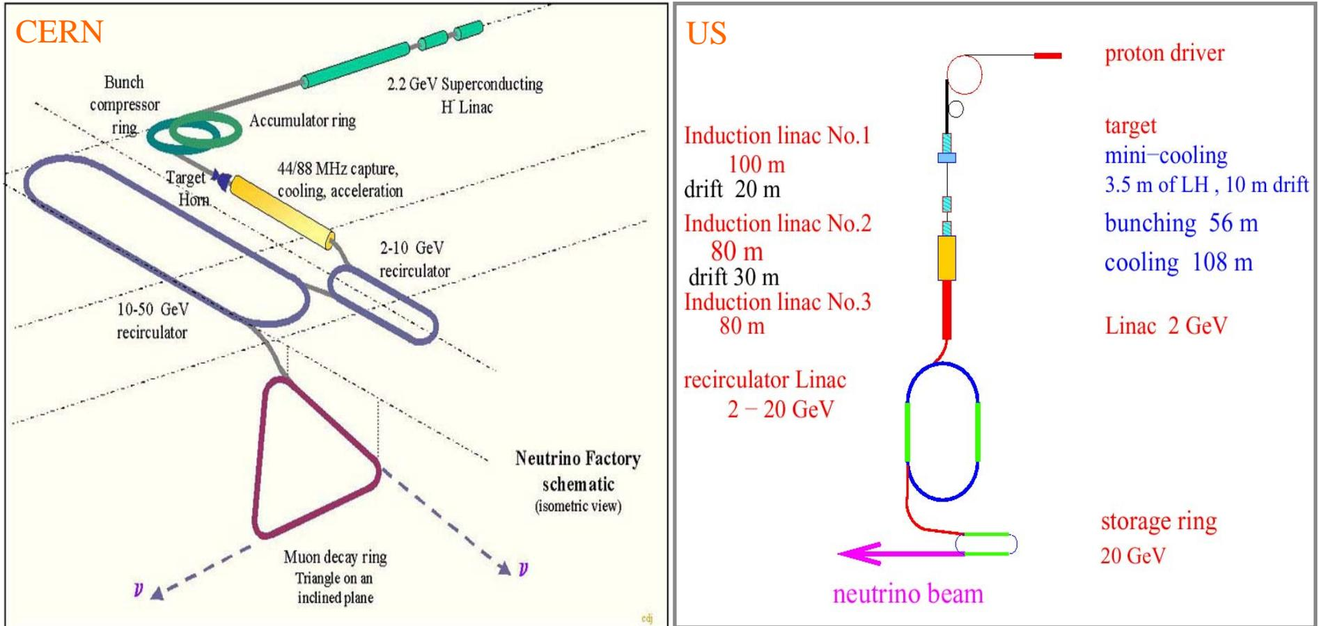
~ MW  $p$  beam  $\rightarrow$  high-power target  $\rightarrow$  pions, focused & decay  $\rightarrow$  muons
