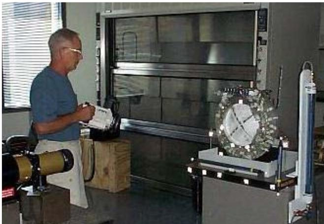
Windows machined w/ integral flange out of single disk of Al alloy
