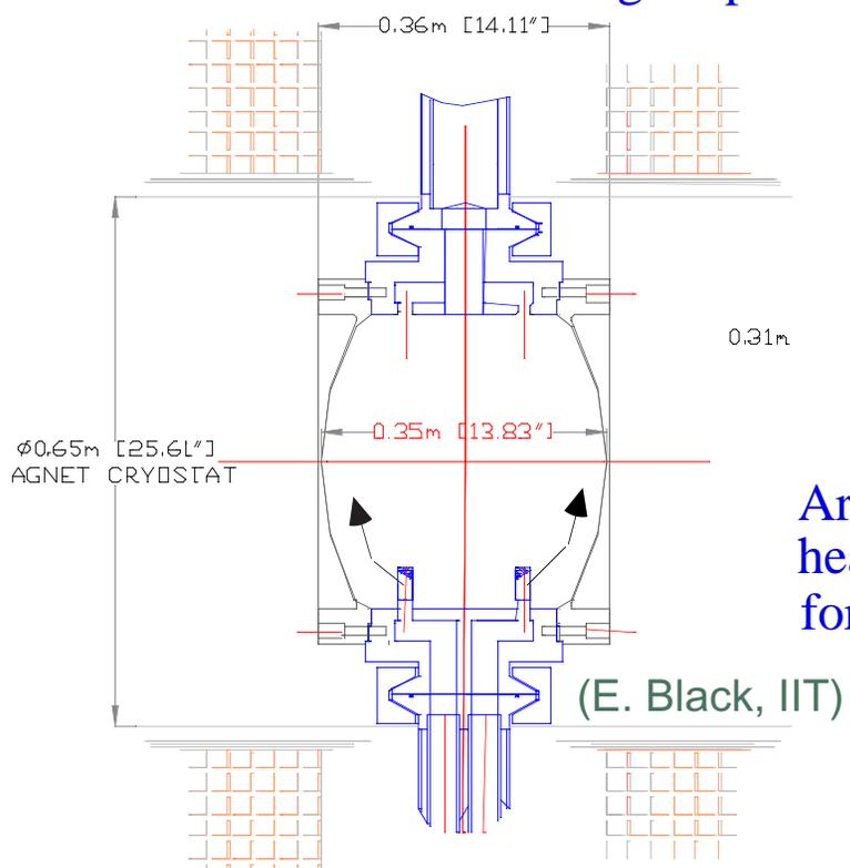
KEK/Osaka: Convection-cooled absorber with internal heat exchanger
