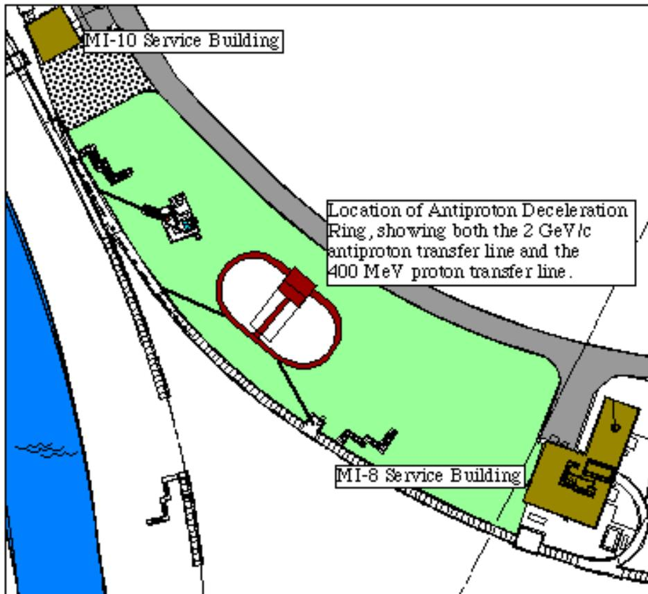
Figure 5: Sketch of the geometry of the antiproton deceleration ring, also showing its antiproton 2 GeV/c transfer line and 400 MeV kinetic energy proton transfer line. The protons are used to commission the ring and allow collider-mode particle physics experiments.
