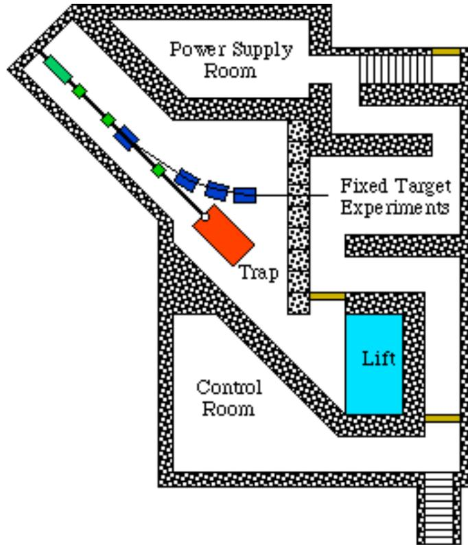
Figure 4: Sketch of the experimental enclosure in which antiprotons are further decelerated via  $dE/dx$  in a degrader. Indicated on the sketch are the Penning trap and a separate experimental area for patient therapy tests and other fixed target studies.
