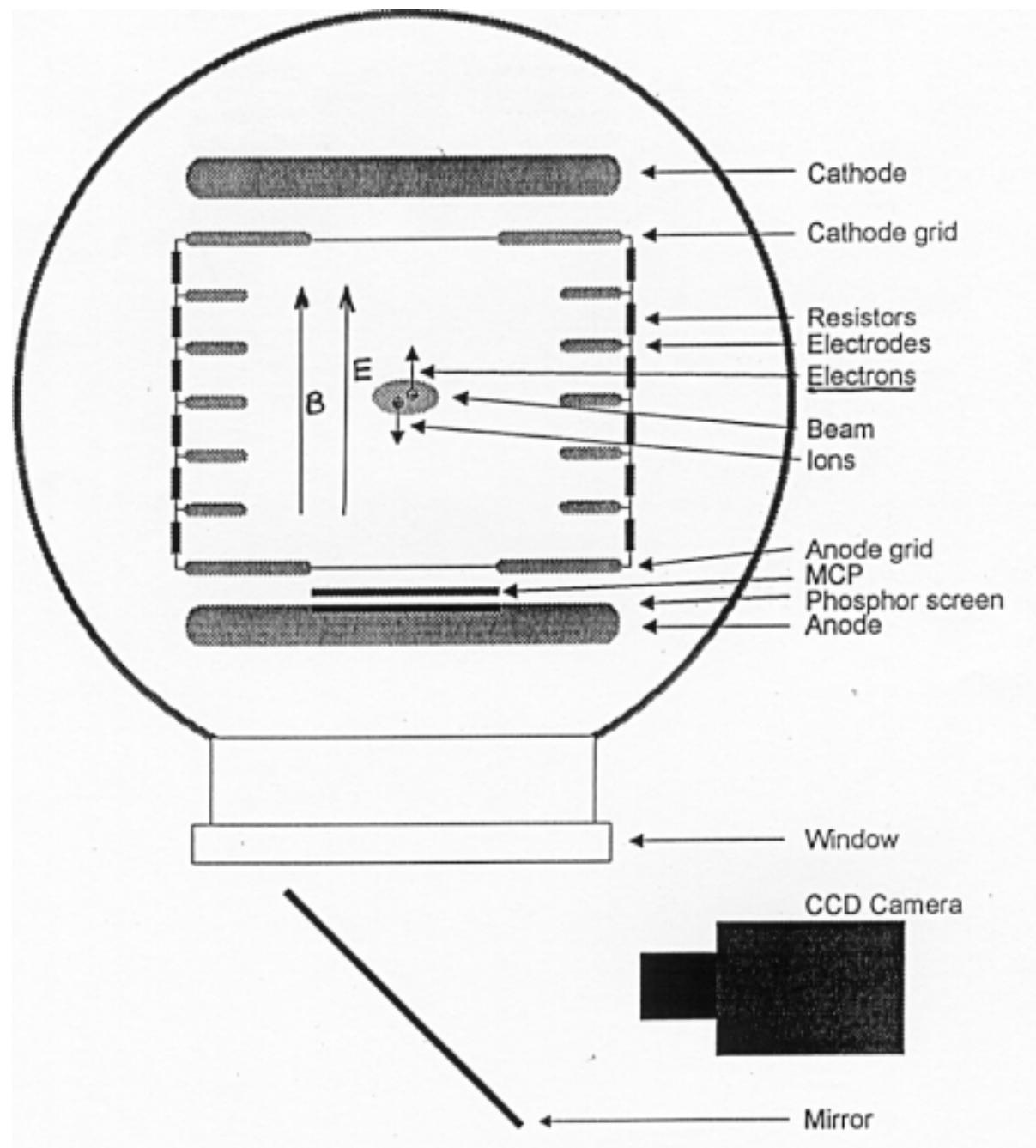
DESY Restgas Ionisation Profile Monitor used at CERN
