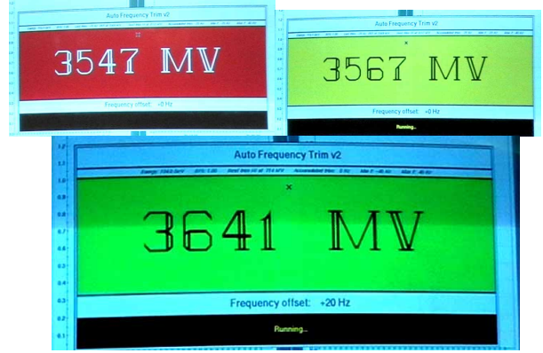
Figure 7: Display output (total RF voltage) of the computer program that automatically controlled J_x . The three cases correspond to 1 klystron off (upper left), recovering (upper right), and all normal (bottom).
