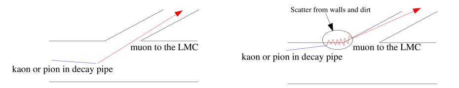
LMC collimator designed to let in clean muons and reject dirt muons.
